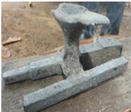
Figure 4. The as-cast grey cast iron-copper alloy.
