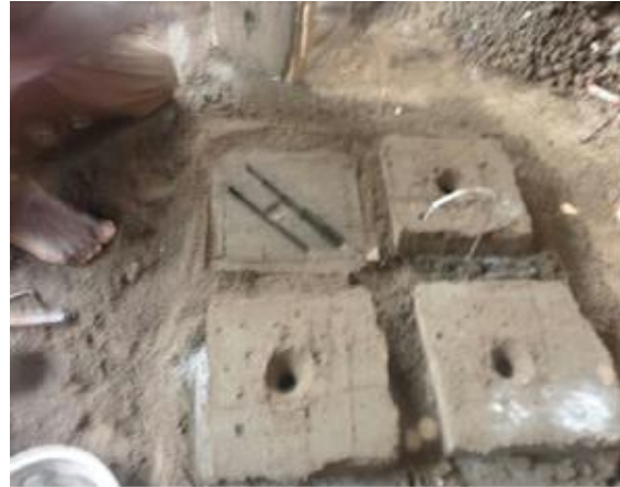
Figure 1. The cope and drag mould.
