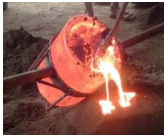
Figure 3. Pouring into mould.
