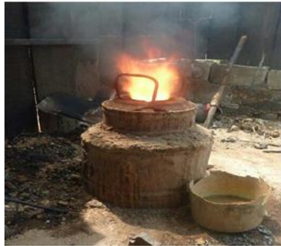
Figure 2. 60 kg crucible furnace.
